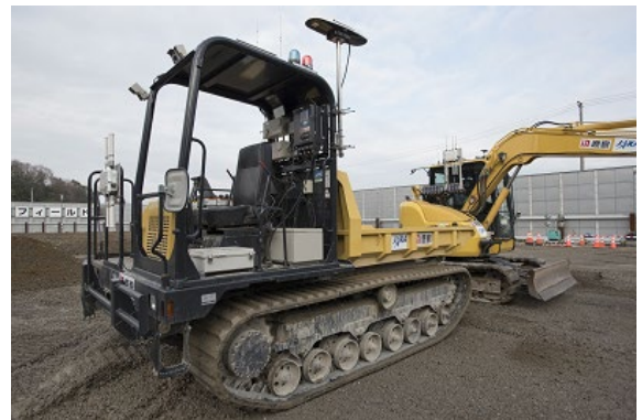
Figure 3 Remote-controlled crawler carrier. A global positioning system (GPS), and a laser range finder were installed on the backhoes and the carrier. The position of the machineries can be estimated while constructing a 3D map of the surrounding environment. Inclinometers were mounted the boom, arm, and bucket of the backhoes to measure their rotation angles.
